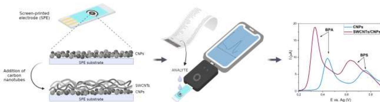
Figure 1. Comparison detection of BPA and BPS by SPE based on carbon nanoparticles and single-wall nanotubes via DPV [3]
